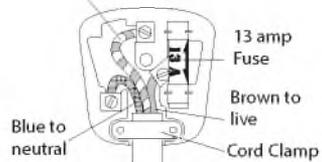
As the colours of the wires in the mains lead of this appliance may not correspond with the coloured markings identifying the terminals in your plug, proceed as follows:
